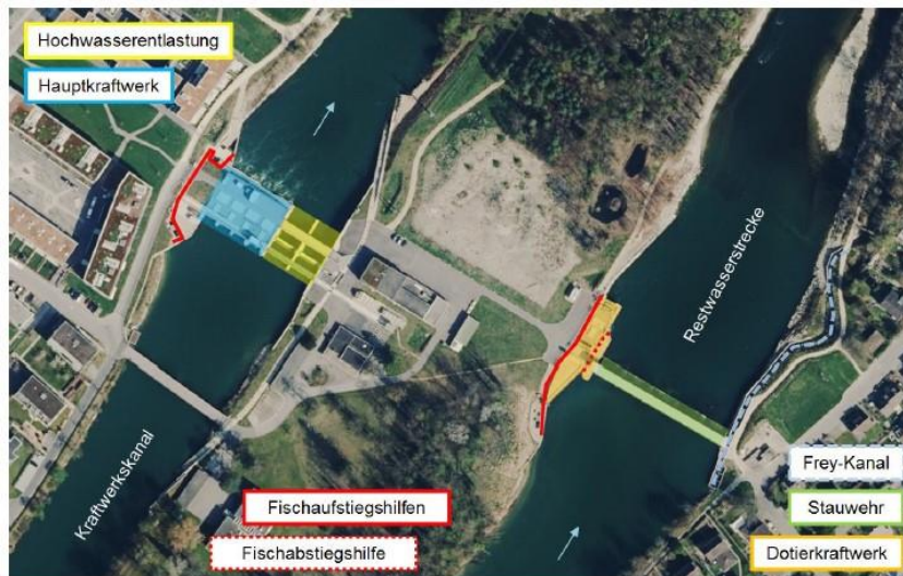
Figure 1. The different sections of Ruchling power plant (ArcGIS, accessed 18 September 2018).
