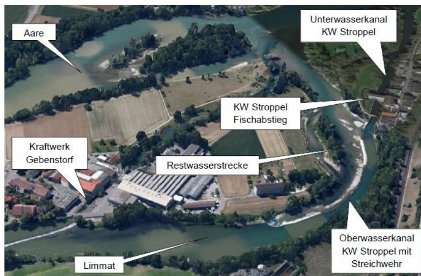
Figure 2. Stoppel small hydropower plant, including Gebenstorf power plant, upstream on the Limmat and Aare rivers (direction of flow from left to right, source Google Earth).
